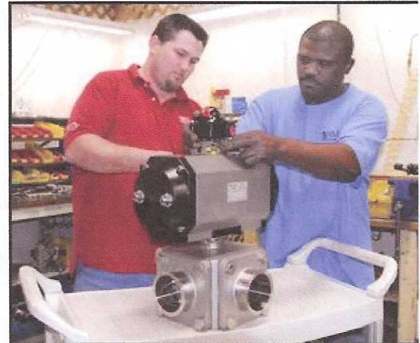
zoom Christopher Hand, left, and Henry McDaniel bench test assembled 4-inch sanitary multi-port Tru-Flo automated valve at Quality Sourced Manufacturing in Easley. ALAN DEVORSEY / Staff
