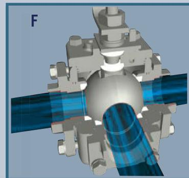
The multiport is designed for applications requiring a 3-way ball valve to close the center port and have the flow go straight through the valve (Fig. D). It allows for a positive seal thus eliminating the need for a common port. The L-port can go from center to left (Fig. E) or center to right. The T-port can do the above configurations in addition to all three ports opened at once (Fig. F).
