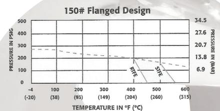
NOTE: Dotted line shows the rating for valve body. Solid line shows the rating for valve seat. Both ratings need to be consulted when determining the limitation of the valve for specific application. Consult factory for other seat material.
