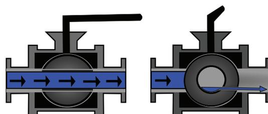
When the valve is open, system fluids flow through the valve. The vent passage allows pressure inside the valve to remain equal to system pressure.
