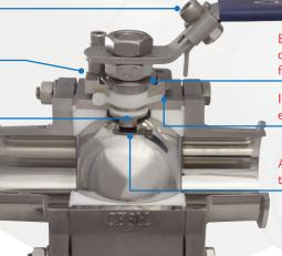
Belleville washer and 3-piece packing design adjusts for wear and temperature fluctuations
